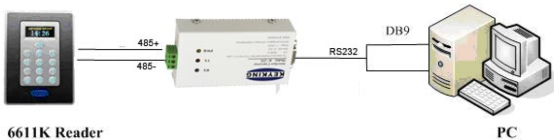
Image #5-3 Diagram for IC-232
